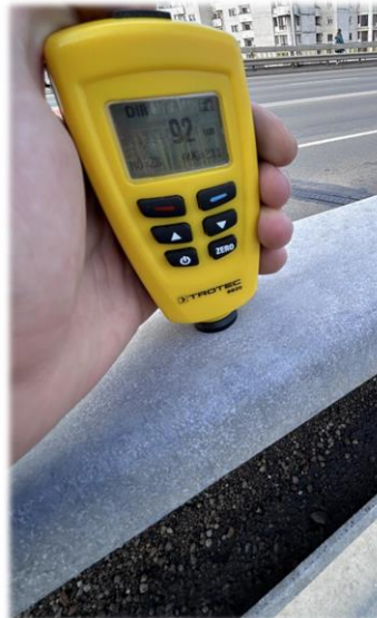
Parapet stradal zincat termic 92 microni
